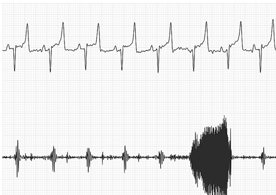
Fig. 2. Example of an artifact on phonocardiographic tracing due to the animal's vocalization.
