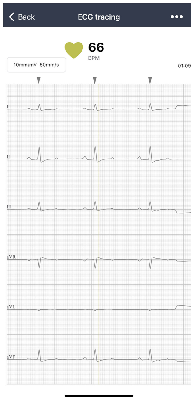
FIGURE 2 Smartphone display during an electrocardiographic (ECG) recording obtained with the smartphone-based ECG device used in this study. Note that all six leads (i.e., leads I, II, III, aVR, aVL and aVF) are simultaneously recorded, with a paper speed of 50 mm/s and a paper sensitivity of 10 mm/mV
